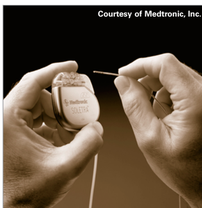
Figure 2. A deep brain stimulator, showing the battery and electrode tip
